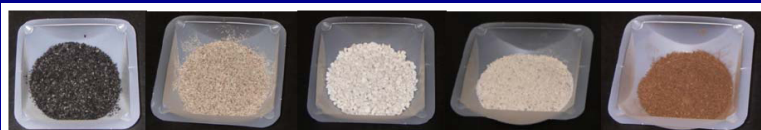
Media (from left to right): GAC, Rhyolite Sand, Site Zeolite, Surface Modified Zeolite, Sphagnum Peat Moss
