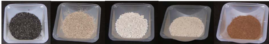
Media (from left to right): GAC, Rhyolite Sand, Site Zeolite, Surface Modified Zeolite, Sphagnum Peat Moss
