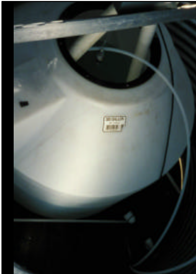
Pilot-Scale Wet Detention Pond used at Lincoln Creek Side-Stream Toxicity Test Facility to Measure Reduction in Toxicity due to Removal of Stormwater Particulates
