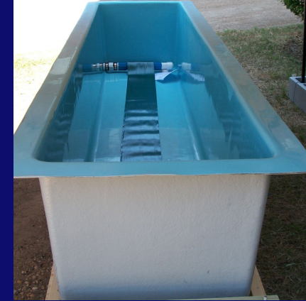
A fiberglass trough 10 ft long and 2 x 2 ft in cross section used as the pilot-scale biofilter
