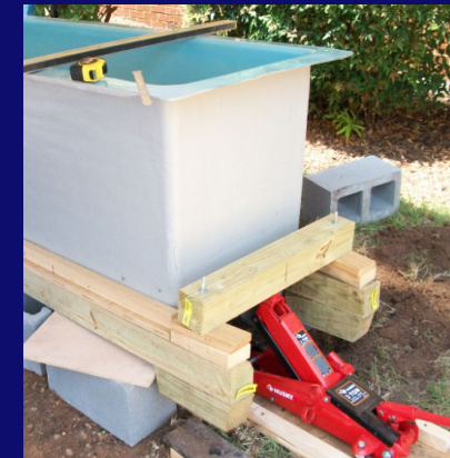
test for effect of length and slope on the drainage characteristics of SmartDrain™ material
