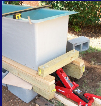
test for effect of length and slope on the drainage characteristics of SmartDrain™ material
