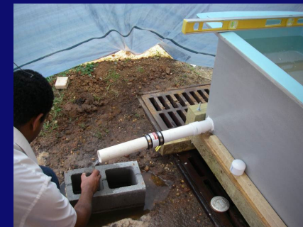
Flow rate measurement from effluent of the biofilter
