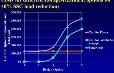
Only the smallest vault with two cartridges is needed. No additional storage is needed. The expected cost is about \$13,000 per acre of impervious acre.
