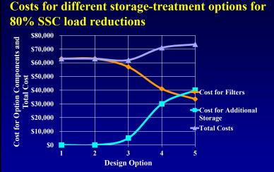
An intermediate control option is slightly more cost-effective. This option uses the large vault with 15 filter cartridges, plus the small vault with 3 more cartridges, at about \$62,000 per impervious acre.
