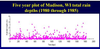
This period was selected by the WI DNR and the USGS to be representative of typical long-term conditions, and not to contain any unusually large rains. The largest rains in this period were about three inches in depth. A treatment system designed to treat 100% of the resultant flows from these events may bypass some limited flows every several years, depending on the frequency of very large drainage-class storm events.
