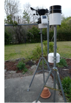
HOBO recording rain gage and Davis weather station surrounded by grass:
