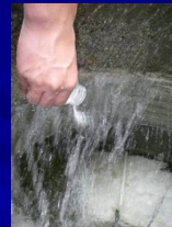
Sediment mixture was manually and consistently added to the influent water over the 30 minute test period.
