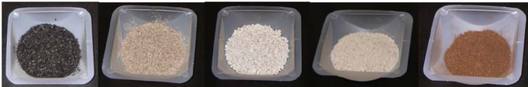
Media (from left to right): GAC, Rhyolite Sand, Site Zeolite, Surface Modified Zeolite, Sphagnum Peat Moss 33
