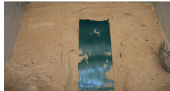
Formica-lined plywood box 1 m by 0.85 m in cross sectional area and 1.2 m tall.
