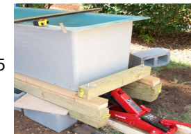
Test for effect of length and slope on the drainage characteristics of SmartDrain™ material
