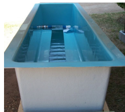
A fiberglass trough 3 m long and 0.6 m X 0.6 m in cross section used as the pilot-scale biofilter
