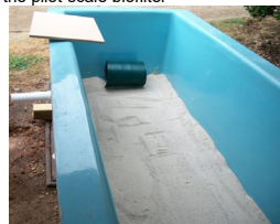
A fiberglass trough 3 m long and 0.6 m X 0.6 m in cross section used as the pilot-scale biofilter
