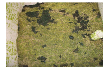
A close-up photograph of algae floating in the tank and trapped on top of the filter sand after the water was completely drained from the tank.
