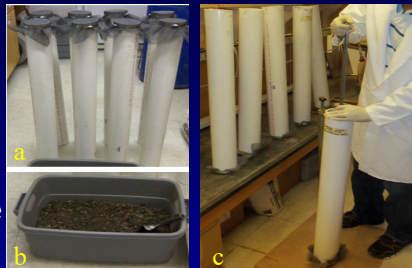
Lab column construction for flow test using biofilter media: a) bottom of the columns secured with a fiberglass window screen, b) biofilter media, and c) compaction
