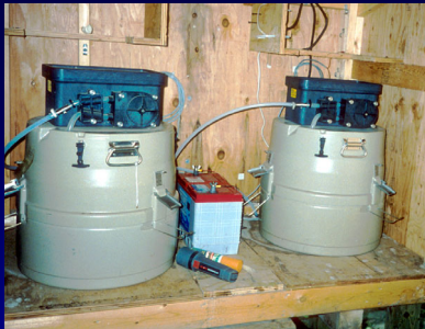
Double monitor setups for sampling over a wide range of flow conditions
