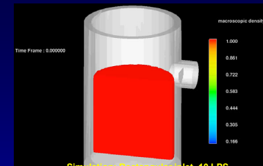
Simulation: Rectangular inlet, 10 LPS Colors represents Density (On calibration process).
