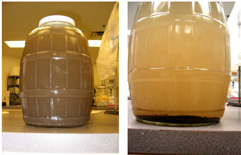
Stirred and Settled Sample, Showing Settleable Solids (Madison high-efficiency street cleaning tests)
