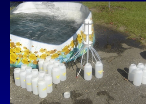
Cone Splitter and Sample Bottles
