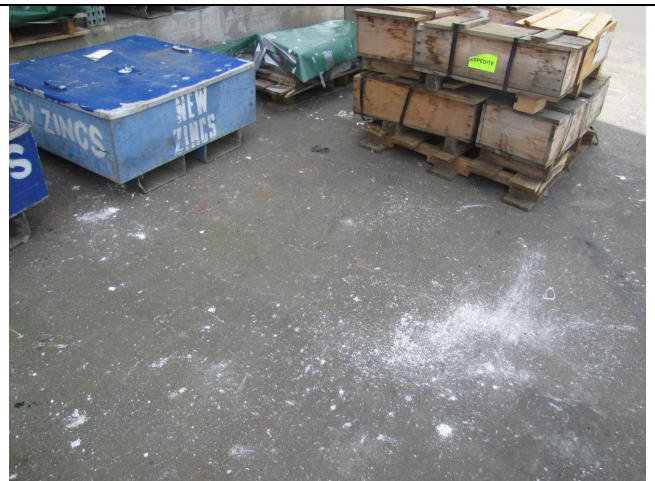
Other galvanized material areas, residue on asphalt is zinc, at naval base.
