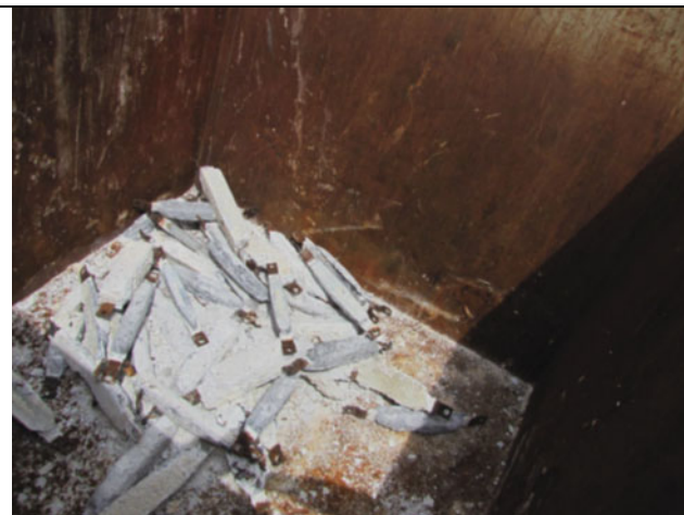
Other galvanized material areas zinc anodes in dumpster, at naval base.
