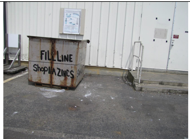
Other galvanized material areas small dumpster with zinc waste. Note zinc particles on asphalt surface, at naval base.
