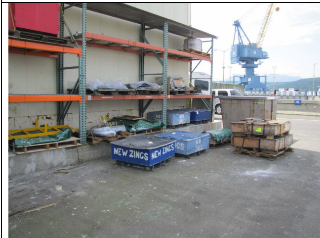
Other galvanized material areas storage and laydown including zinc anodes (note corroded anode material on ground), at naval base.
