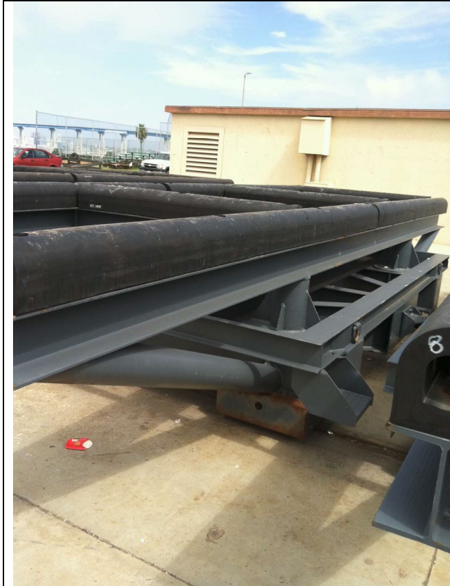
Medium laydown area, painted metal platform supports with rubber (on concrete) at naval base
