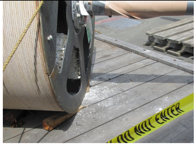
Other galvanized material areas cable reel, note zinc particles from corroded anodes, at naval base.
