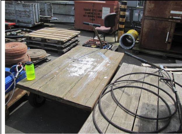
Other galvanized material areas laydown area with miscellaneous items (note zinc debris on table), at naval base.
