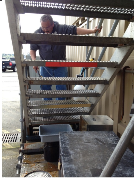
Washdown sampling of galvanized stair steps.
