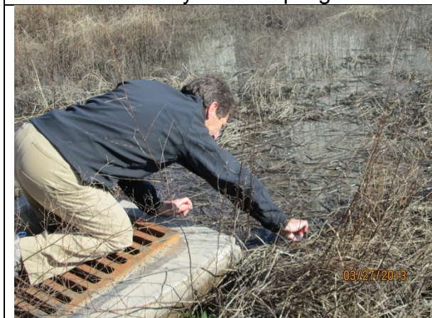
Sampling of accumulated sediment near inlet.
