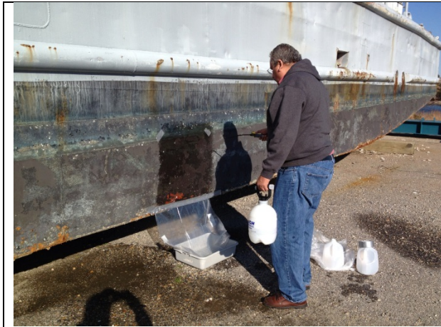
Washdown setups showing sprayer, plastic sheet below target area and plastic tray to capture washdown water (barge hull).
