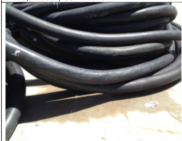
Cables, electrical 3 in. diameter; Pt. Loma Subase
