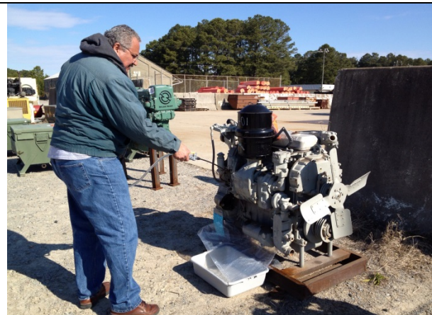
Washdown sampling for engine block.
