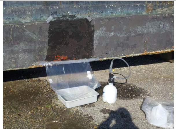
Washdown setups showing sprayer, plastic sheet below target area and plastic tray to capture washdown water (barge hull).
