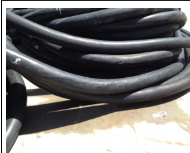
Figure 7: Cables, electrical, black, 3 in. diameter
