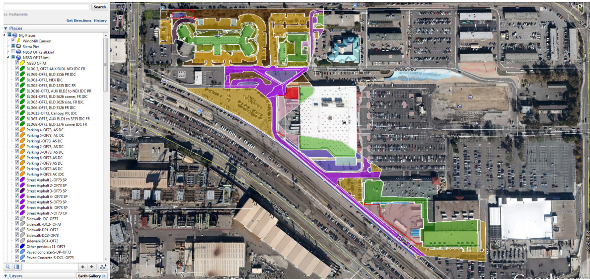
Figure 14. Example of general land use categories placed as polygon overlays in an aerial image generated in Google Earth™. The individual areas of each polygon can be calculated using Free Map Tools. The individual or summed area data for each land use category are entered into the spreadsheet tool.
