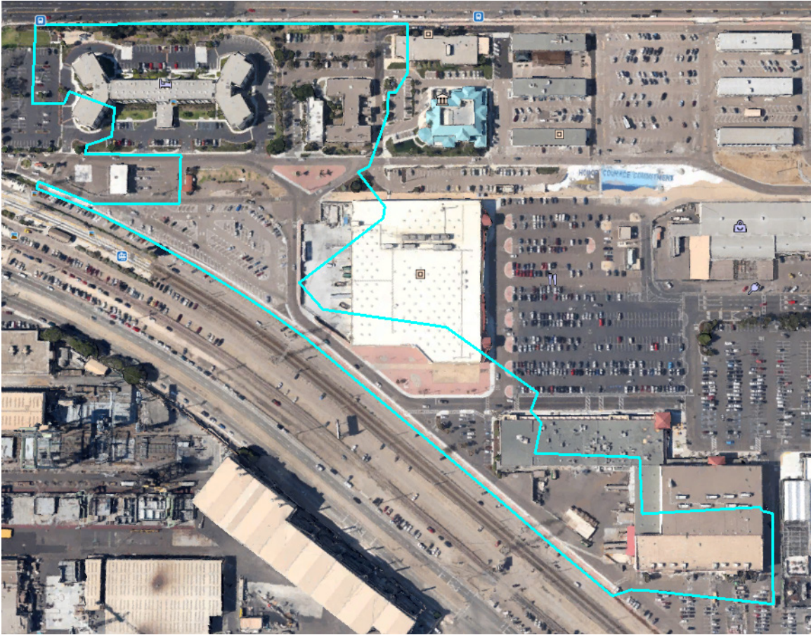
Figure 5. Example outline of Naval Base San Diego storm-water drainage area for outfall 73 using Google Earth™ aerial image as the starting point. The overlay can be facilitated using Google Earth's™ image overlay capability. This complete overview should be printed for use during the site survey, if available.
