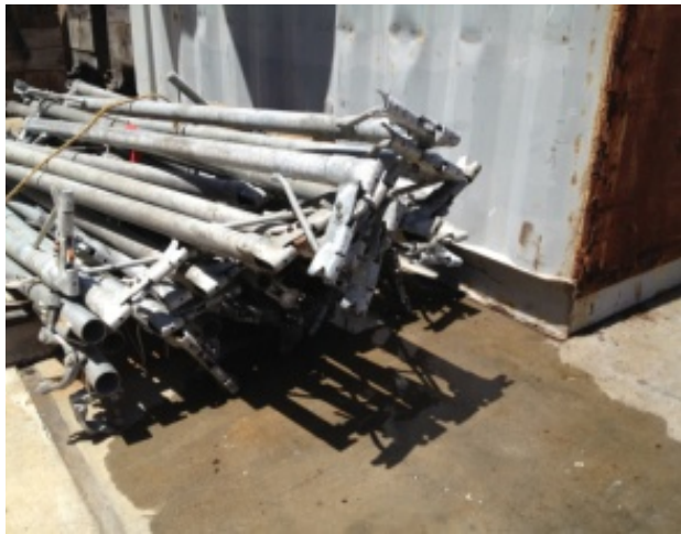
Figure 27: Galvanized scaffold parts
