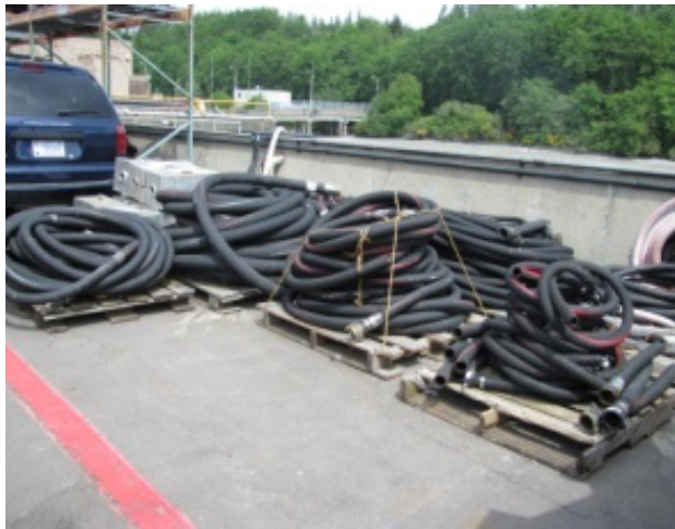
Figure 35: Hose, black, 4 in. diameter
