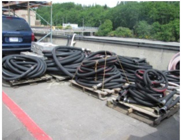
Figure 36: Hose, red, 1.75 in. diameter
