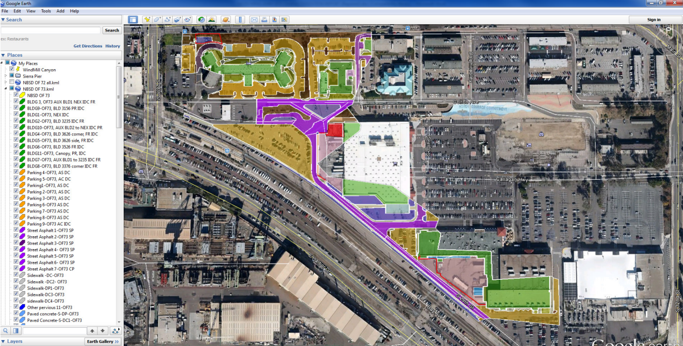
Figure 36. Completed Characterization Polygon View of NBSD OF73, note file names and different polygon colors for different landuse types to the left of the aerial image.
