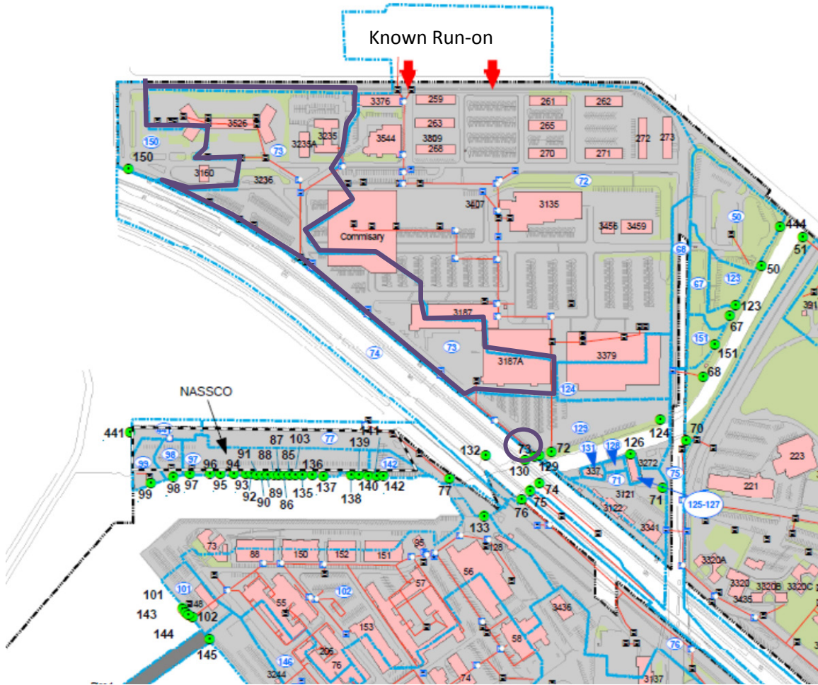
Figure 4. Example outline of Naval Base San Diego storm-water drainage area for outfall 73 (purple outline) using the base's storm-water GIS as the starting point. Red lines show the location of the storm-water conveyance system within each drainage. This complete overview should be printed for use during the site survey, if available.
