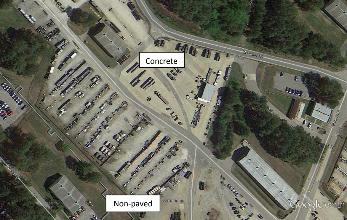
Figure 10. Examples of large surface areas that may not be discernable as non-paved or paved from an aerial image.
