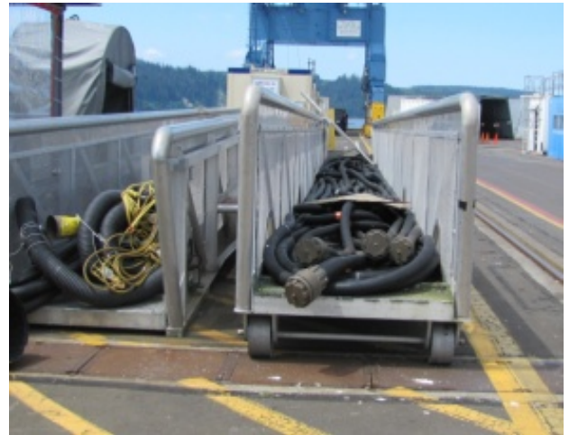
Figure 6: Cable, black, 4 in. diameter
