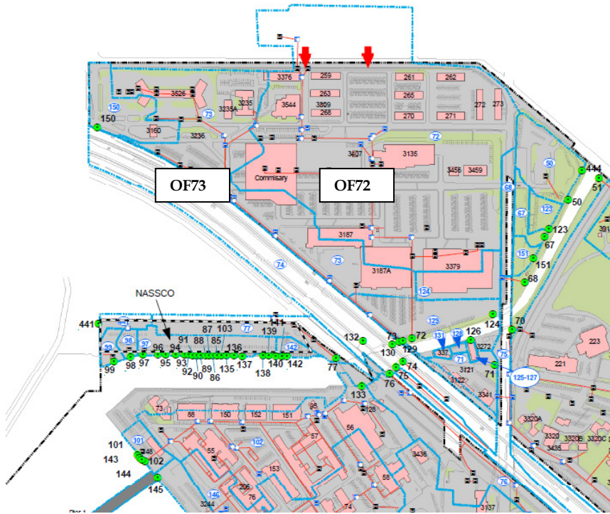
Figure 2. Example of Portion of Facility drawing showing outfall boundaries. This Image shows NBSD OF 72 and 73, along with a portion of OF 51. Blue lines indicate outline boundaries
