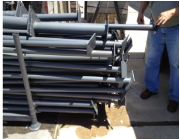
Figure 44: Pipe supports, coated, brown
