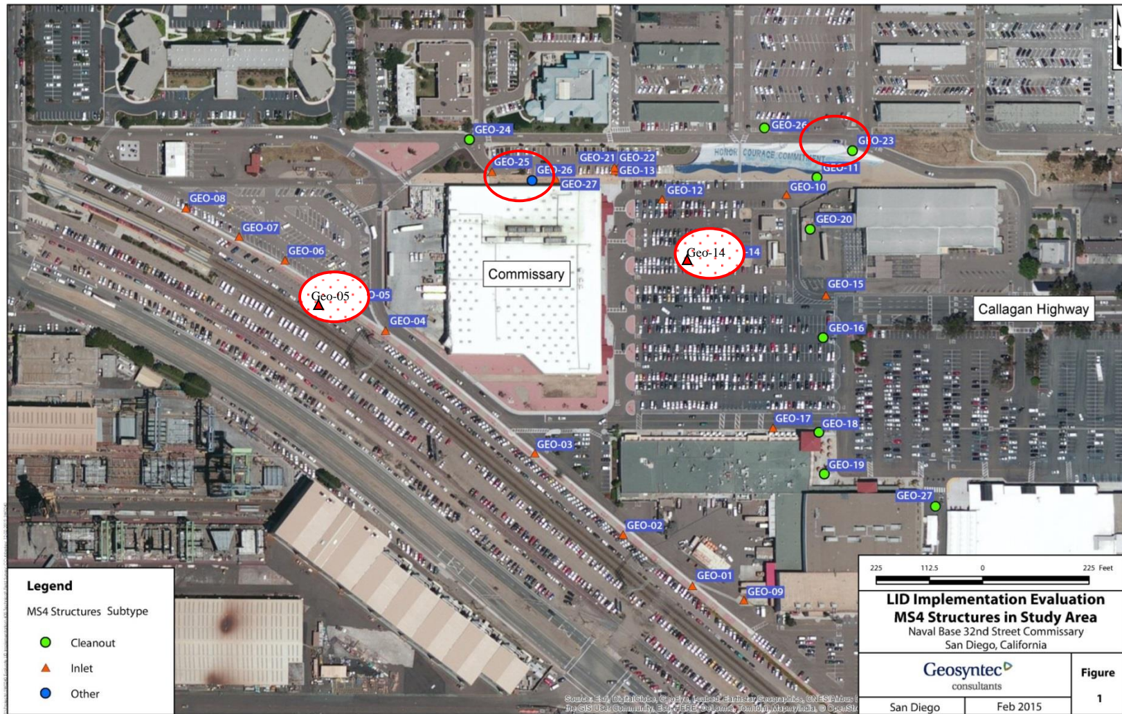
Figure 3. Potential locations identified for LID technology implementation. The four red-circled locations were downselected using criteria shown in Table 1. The two filled in circles identify the final sub-drainages chosen for demonstration. Aerial photo supplied by Google Earth.
