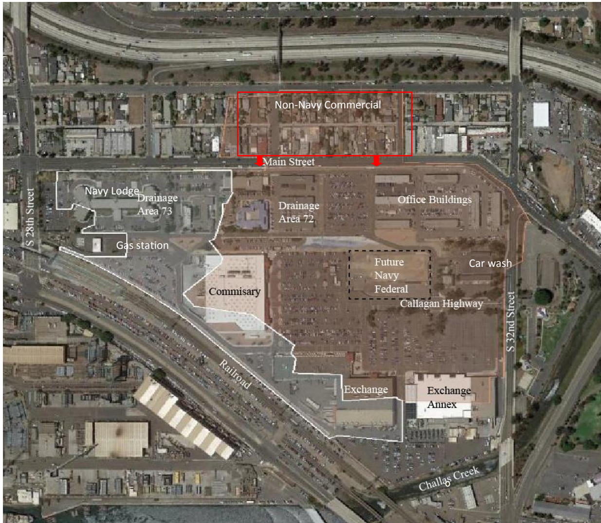
Figure 1. Commercial area of NBSD used for the LID demonstration project. The area is composed of two main stormwater drainage areas (outlined in white and beige) both discharging to Chollas Creek at the southeast corner of the property. The area outlined in red is composed of non-Navy commercial properties potentially discharging on to the base. Aerial photo supplied by Google Earth.
