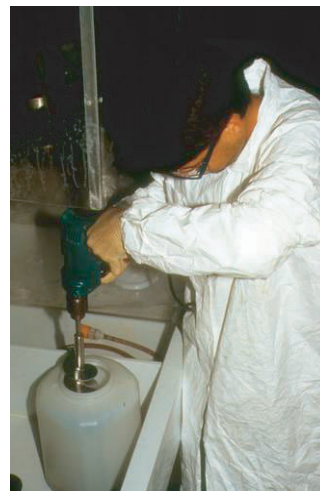
Figure 5.78 Mixing sediment with a drill auger.
