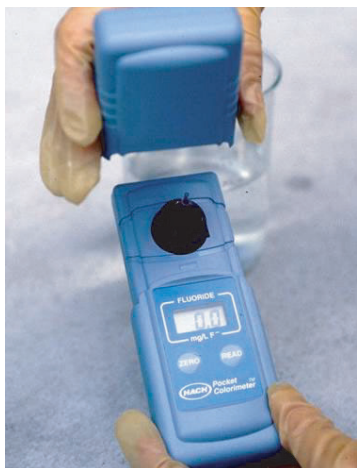
Figure E.7 Reading AccuVac absorbance.
