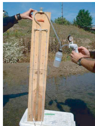
Figure 5.94 Field manometer connected to mini-piezometer to measure vertical flow through sediments.
