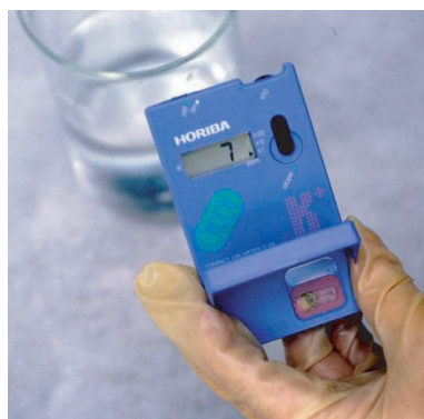
Figure 6.94 Horiba Cardy ion selection electrode for potassium.
