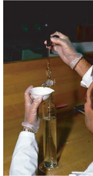
Figure 6.104 Andreason pipette for particle size determinations.
