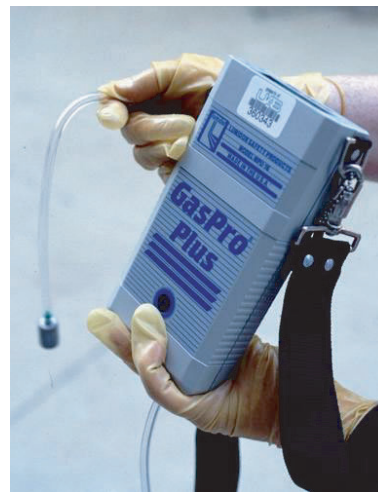
Figure 6.114 Portable gas analyzer for H 2 S and explosive conditions.
