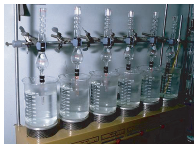
Figure E.21 Alternative micro Kuderna–Danish concentration method.
