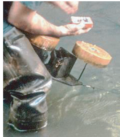
Figure 6.121 Diatometer for artificial substrate periphyton sampling.
