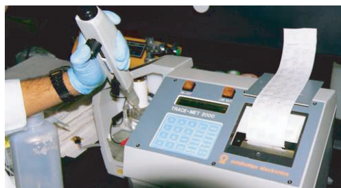
Figure E.11 Anodic stripping voltammeter (Outokumpu) for heavy metal analyses.
