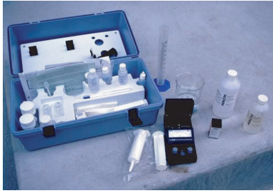
Figure 6.78 HACH LeadTrak field test kit.
