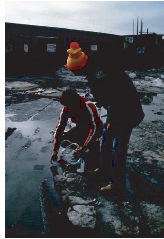
Figure 5.48 Sheetflow sampler being used to sample snowmelt.
