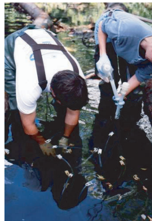
Figure 6.169 Loading in situ chambers that are peepers for sediment–water interface exposures.
