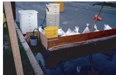
Figure 5.53. Runoff collection area for Toronto washoff tests.
