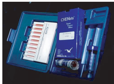
Figure E.8 CHEMetrics nitrate test kit.
