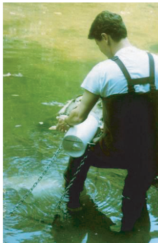
Figure 4.49 Placement of in situ pathogen die-off test chambers in Five-Mile Creek. (Courtesy of John Easton.)
