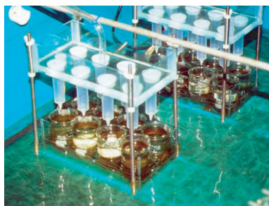
Figure 6.149 EPA whole sediment, overlying water renewal design.
