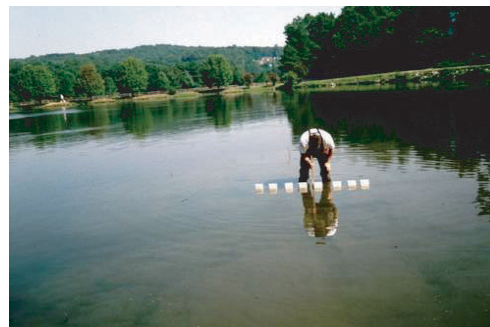
Figure 5.83 Ten replicate high-resolution peepers (to obtain larger water composite samples).
