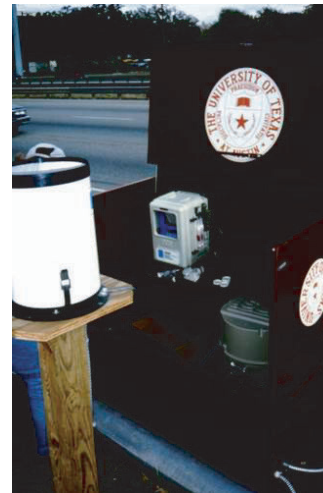
Figure 5.56. Sampler and flow monitoring equipment at Austin freeway washoff test site.
