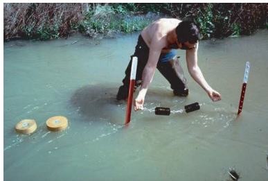
Figure 4.9 Artificial substrate sampling using a Hester-Dendy multiplate sampler in Coyote Creek.
