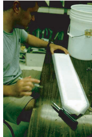
Figure 5.81 Small-volume peeper assembly showing 75- \mu m nylon screening.
