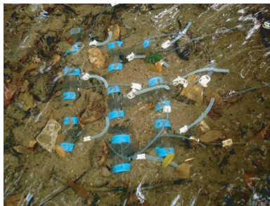
Figure 6.166 In situ sediment–water interface chambers buried.
