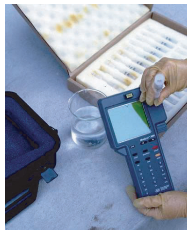
Figure 6.80 Metalyzer 3000 metals analyzer.
