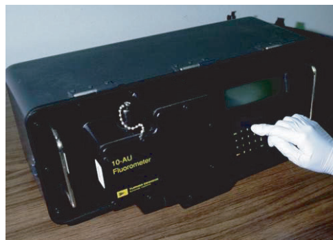
Figure 6.10 Current model Turner 10-AU fluorometer being calibrated in the laboratory before field deployment.
