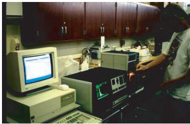
Figure 6.102 Coulter Multisizer for stormwater particle size analyses.
