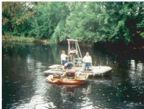
Figure 5.70 Shallow water vibratory core collection.
