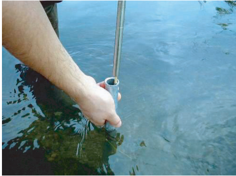
Figure 5.92 Placement of mini-piezometers into support tubing.
