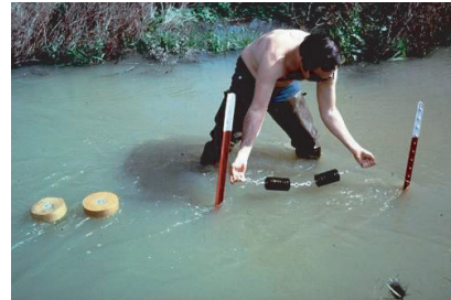
Figure 6.127 Periphyton sampler in place, plus Hester-Dendy samplers.
