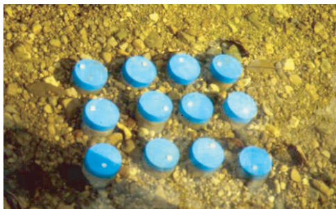
Figure 6.168 Chambers for conducting sediment bioaccumulation studies.
