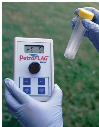
Figure 6.76 Sample being read using PetroFlag.
