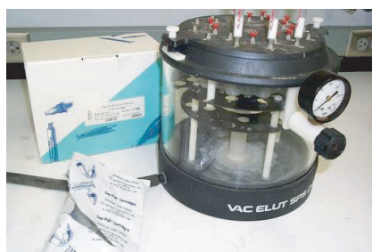
Figure 6.109 Solid phase extraction manifold for resin exchange experiments.
