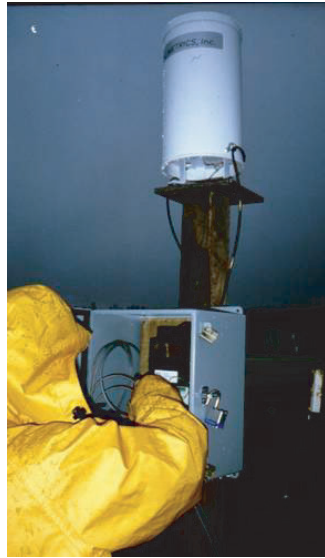
Figure 6.20 Tipping bucket rain gauge with data logger.
