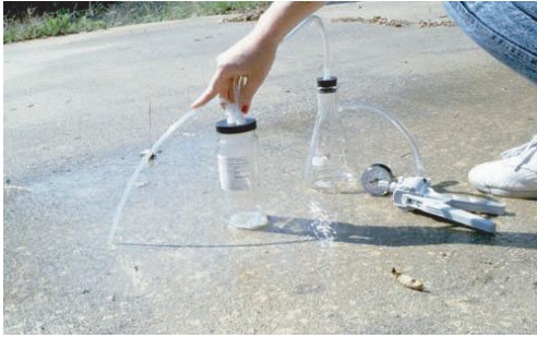
Figure 5.47 Sheetflow sampler operated by hand vacuum pump.
