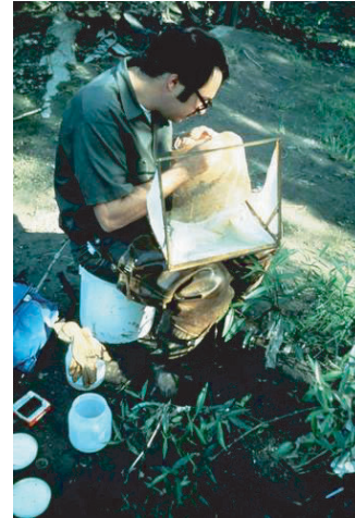
Figure 4.8 Removing benthic macroinvertebrate samples from Surber sampler.
