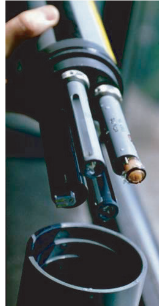
Figure 6.69 YSI 6000 sonde detail showing several probes.
