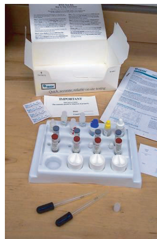
Figure 6.77 Dtech Immunoassay test kit for BTEX.
