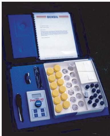
Figure 6.75 PetroFlag kit for field analyses of BTEX.
