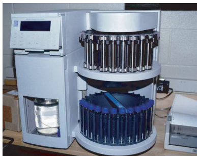
Figure E.23 Dionex ASE for automatic extractions of organics from sediment samples.
