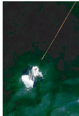
Figure 6.59 Underwater Secchi disk showing slow disappearance of contrasting disk sectors.
