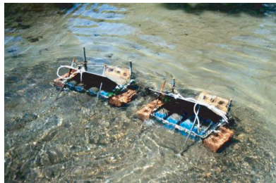
Figure 6.163 In situ chambers with water or sediment exposures with high-flow deflector.
