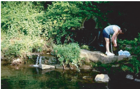
Figure 6.113 Collecting outfall samples for inappropriate discharge evaluations.
