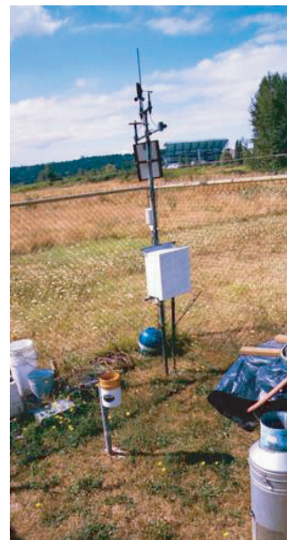
Figure 6.36 Weather station at UW soil infiltration test plot.
