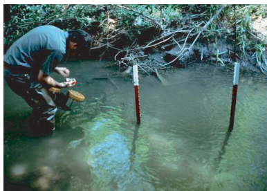
Figure 4.11 Artificial substrate diatometer sampler being loaded with glass microscope slides in Coyote Creek.
