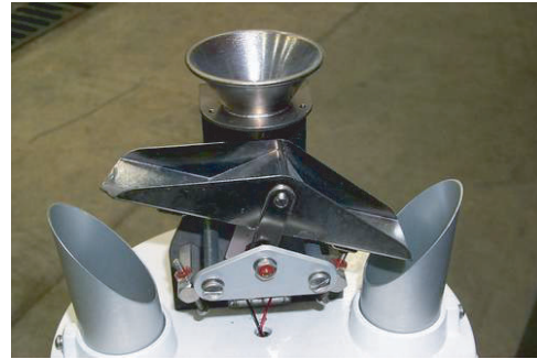
Figure 6.21 Close-up of tipping bucket rain gauge mechanism.
