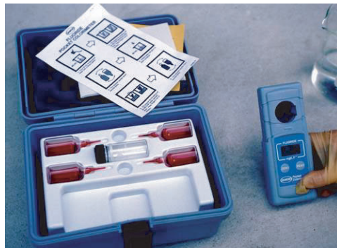
Figure E.6 HACH AccuVac kit for fluoride.
