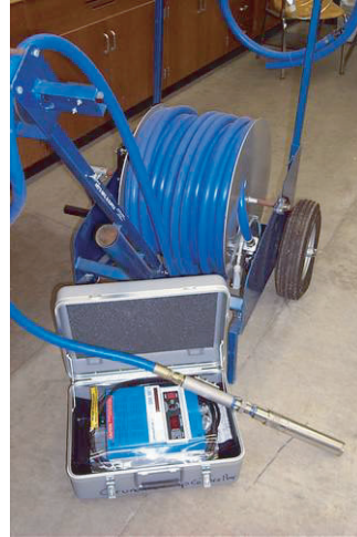
Figure 5.40 Grundfos Redi-Flo2 pump sampler with controller.
