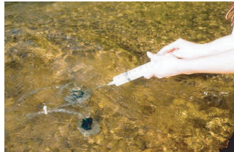
Figure 5.85 Withdrawing interstitial water sample from large-volume peeper.
