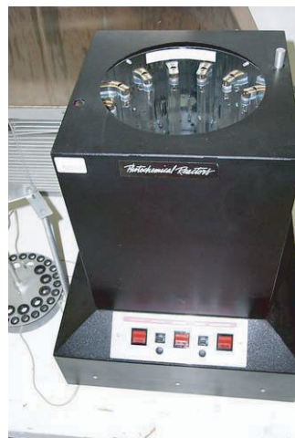
Figure 6.108 UV light digestion for controlled photo-oxidation.
