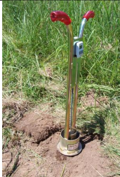
Turf-Tec infiltrometer at bare soil location.
