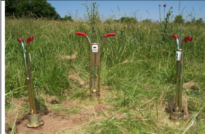
Set of three Turf-Tec infiltrometers for infiltration measurements in pre-development soils.
