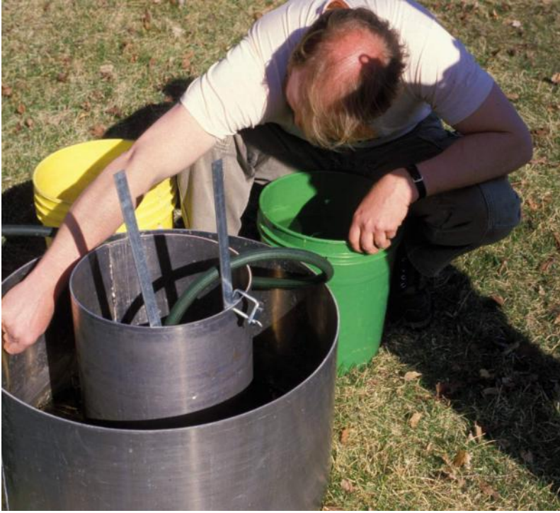
Traditional ASCE double-ring infiltrometer.
