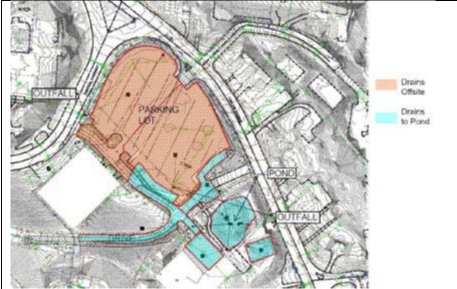
Drainage Areas Pre Construction
