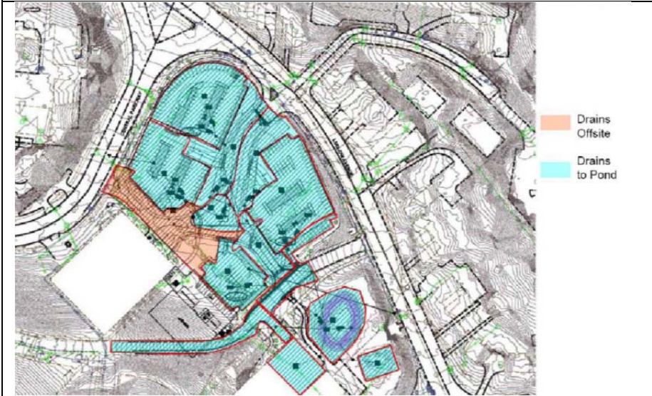
Drainage Areas Post Construction
