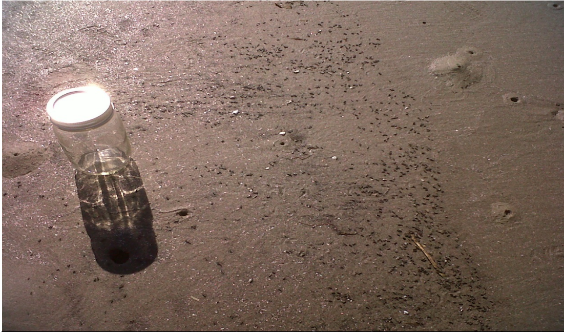
Figure 6-28. First available access to the marine (Gulf) waterfront (terminus of security fence easily visible to the northeast from this location). Site of Sample-3, very dark gray, sprinkles appeared to be actively washing ashore in (calm) surf. Sprinkles were slick/sticky but not gritty when ground between fingers. Sample-3 included a few “brown gobs” (slick/greasy*, but with incorporated sandy texture, visually more like what was described as weathered tar balls on TV) that were intimately co-located. Sample-2 was also taken near here (directly up-gradient) above the apparent high-tide line (well dried rind, smelled distinctly of hydrocarbon when broken, but nothing but sticky inside). [*slick/greasy - little friction when rubbed (except for obvious sand), little resistance to pulling fingers apart]
