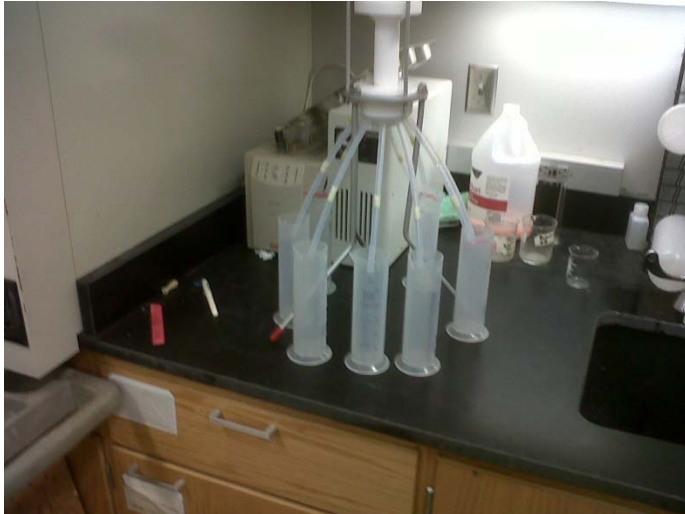
Figure 2-21. Cone splitter for further sample splitting.
