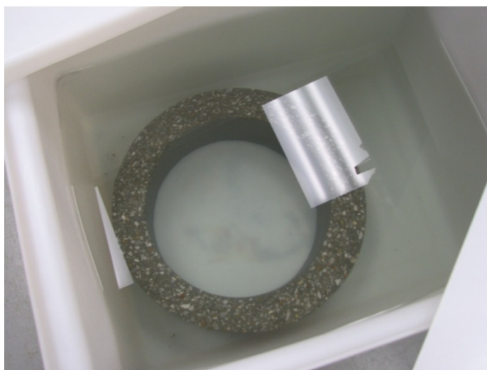
Figure 3-7. Concrete pipe sample submerged in test solution.
