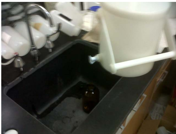
Figure 2-20. Churn splitter for initial sample splitting into large portions.
