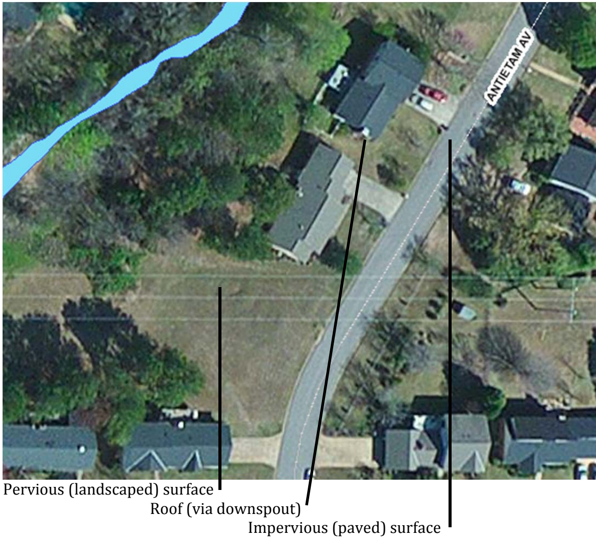
Figure 2-17. Academy Drive residential area sheetflow monitoring locations.
