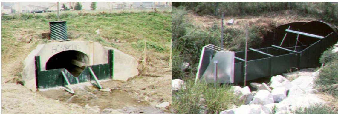
Figure 1. Example outfall monitoring with V-notch weir and flume set-up. (photo courtesy City of Baltimore, MD)
