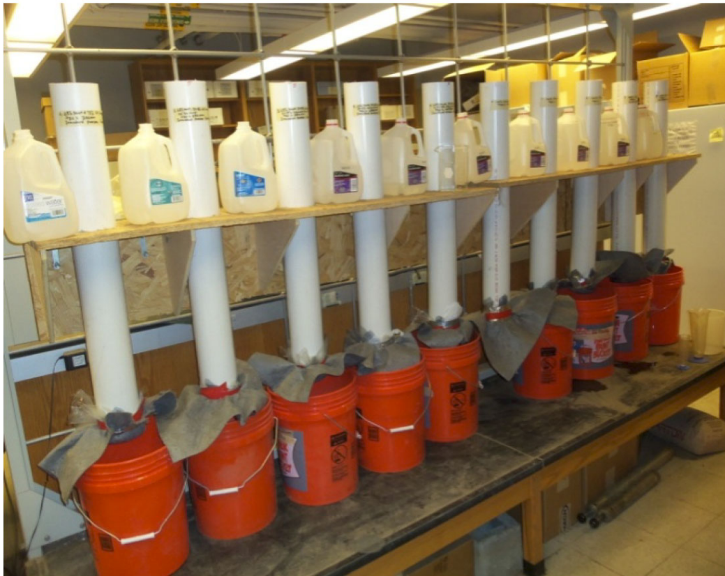
Figure 113. Laboratory Column Setup for Infiltration Measurements.
