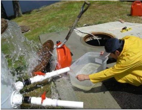
Pumped river water is discharged from splitter barrel to the 11 gallon plastic tray to manually measure the flow entering the Up-Flo® Filter
