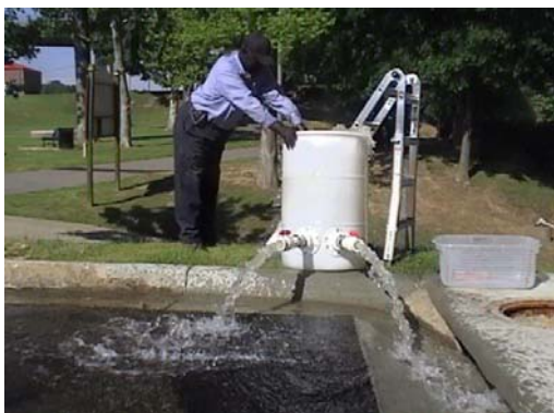
River water is pumped into the plastic flow splitter barrel (high flow test)
