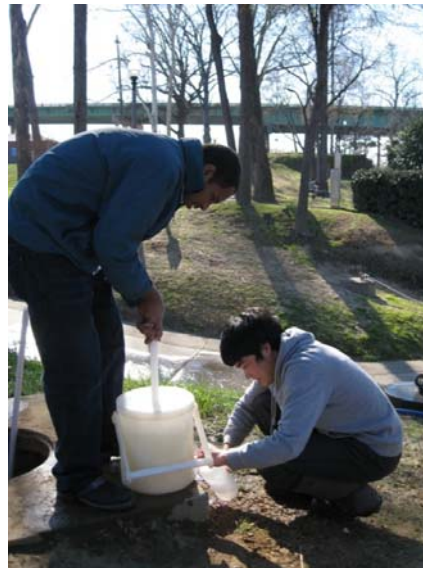
Sample splitting using churn splitter
