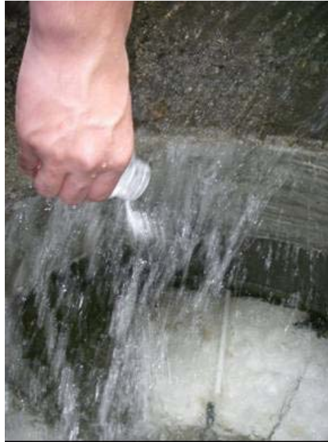
Sediment mixture is added to the flow entering the Up-Flo® Filter
